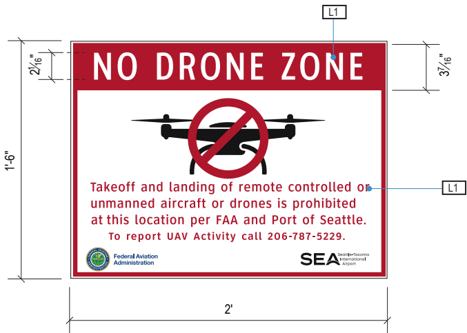
5-RG.03 No Drone Zone - High Intensity Reflective 0.063 Aluminum Substrait - White/Red Background with Red/White Legend - Digital Print FAA Symbol
