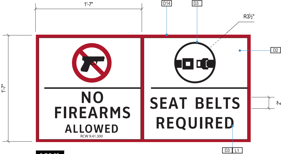
2-RG.05 Seatbelts and No Firearms - High Intensity Reflective 0.063 Aluminum Substrait - White background with Black Legend
