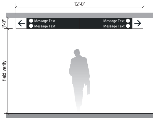
3-DR.11 Overhead Directional - 2 directions / 1-2 messages per direction - 2 Sides
